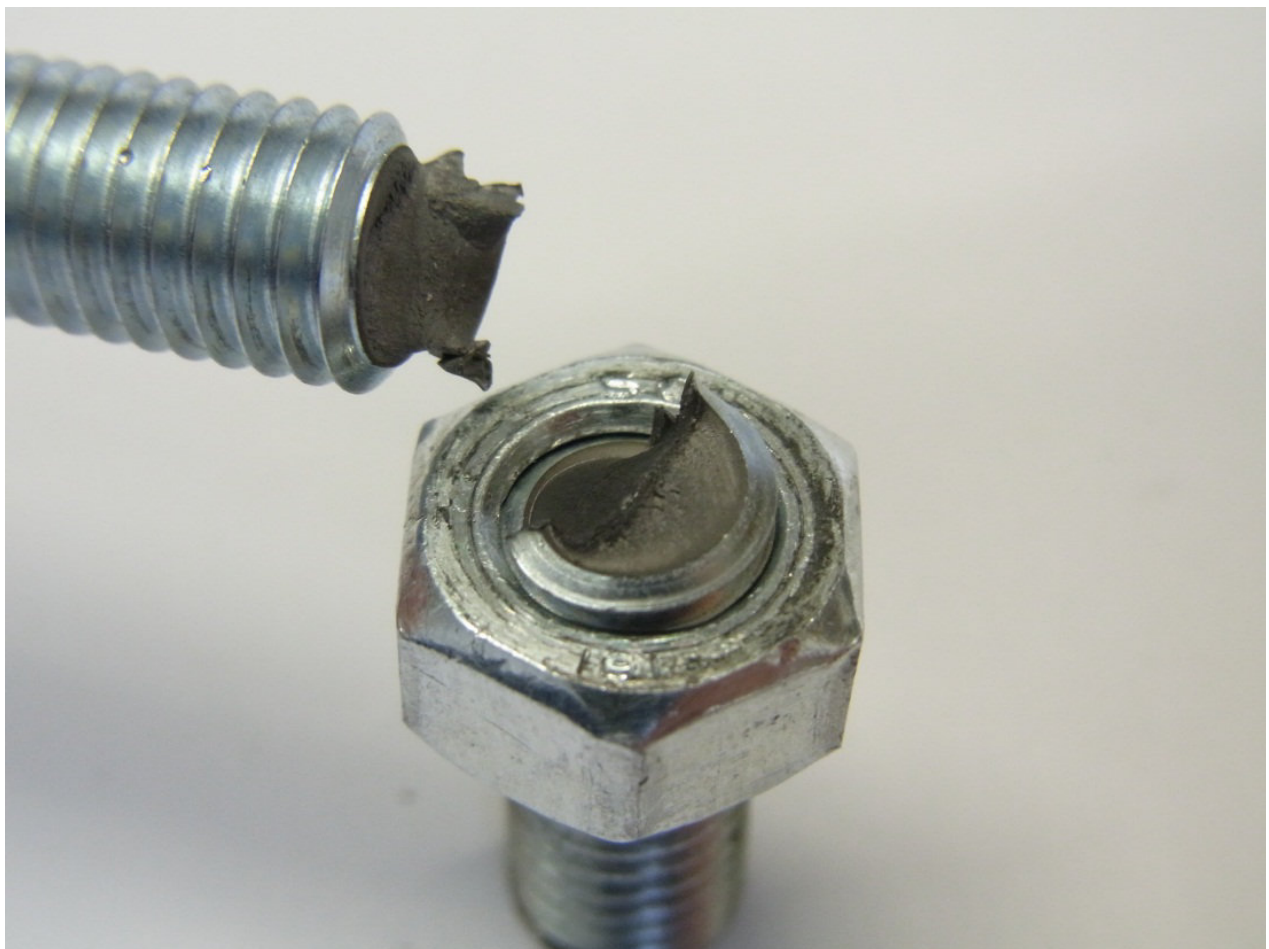
Figure 6: Fatigue failure of a threaded stud M8-8.8 in first carrying pitch
